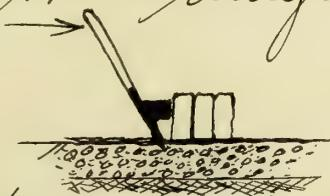
Some such treatment would undoubtedly secure a more rigid pavement and reduce the size of the joints considerably over that now secured in such pavements. The blocks are too heavy for a single man to place with a good bearing one against another.
